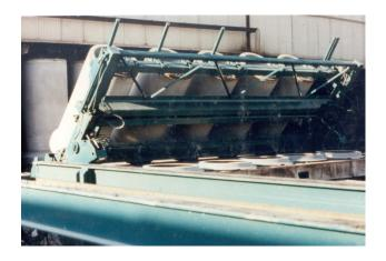
Multiple pipe tipping systems are engineered to work with moving floor systems up to 20'-0" wide. The tippers are operated manually. Once tipped the pipe are transferred to an off load table via the built-in conveyor system. Systems are designed for pipe up to 48" in diameter. All tippers are designed to the same rugged performance standards that are expected from all ERMC products.
