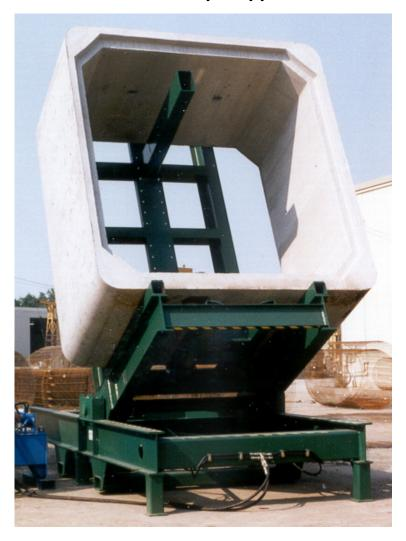
The single station tipper is made to tip box culverts or large diameter pipe without damaging the joint area which reduces the need for repair due to handling.
