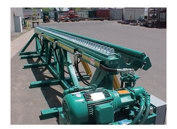
ERMC 180-Degree Single Direction benders have been designed and built to bend D-32 (5/8" WWR) on 4" centers for a full thirty feet.
