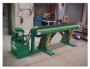
ERMC Single Direction Benders are equipped with individual bending anvils adjustable to bend variable spaced mesh. The typical anvil radius furnished with the bender is <sup>3</sup>/<sub>4</sub>", however, other radii may be furnished by request up to 2.5". Anvils are furnished at 4" spacing
