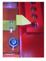
Cam followers accurately guide the moveable beams as you adjust the **Pipe Certa-Fire** for the next test.
