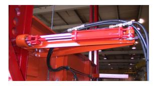
Hydraulic beam lifting and Hydraulic Pinning allow you to quickly and easily change from one pipe size to the next.
