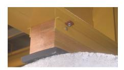
Bell-end pipe present a special challenge. We've made it easy with adjustable top and bottom beams. You can shift the beams to the correct positions to insure the specified loading is achieved.
