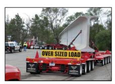
6-Axle Hydra-Steer Tri-Steer trailer with pin on tag axle and pusher axle. Capable of *Crab* steering mode when the tongue is attached to the bridge beam. When tongue is detached from the beam, *Hinge*, and *Front* steering modes can be used.
