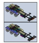
6-Axle Hydra-Steer Tri-Steer trailer with (2) 3 axle upper frames with power units, capability of (1) 6-axle trailer or converting into (2) three axle trailers. The 6-axle trailer has the Tri-Steer capabilities and the 3-axle trailers will only function in the *Crab* steer mode.
