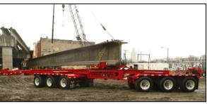
6-Axle Hydra-Steer Tri-Steer trailer capable of *Crab* steering mode when the tongue is attached to the bridge beam. When tongue is detached from the beam, *Hinge*, and *Front* steering modes can be used.
