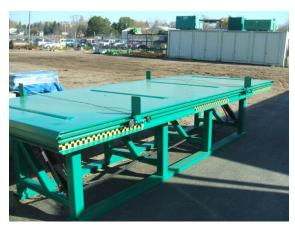
Photos illustrate heavy construction, hydraulic tipping cylinders and table mounted rollers
