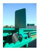
Bumpers are removable and adjustable to include precise bending locations
