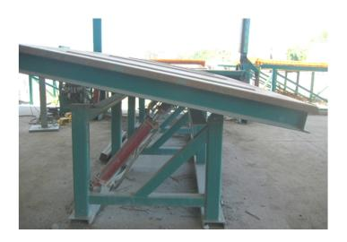
ERMC Tilt Table secures the bent cage safely and securely; then lowers to the floor in the upright position
