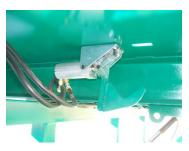
Pneumatic hooks secure the bent mat prior to tilting safely to the floor. In a single 15' table two hooks are standard
