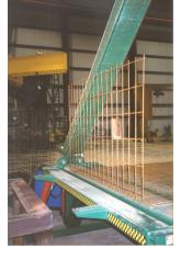
"L" shaped mat is pulled forward and the second bend located
