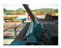
Mat is introduced between the deck and mandrel; and located for the first bend
