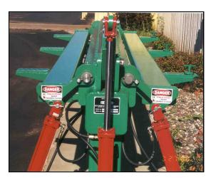
Unobstructed bending deck. Complete "U" shaped cage without removing or turning the mat
