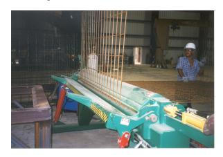
The cage is extracted from the bender by simply raising the mandrel to the full 90-degree position. The arm will completely clear the bending deck for easy removal of the cage.
