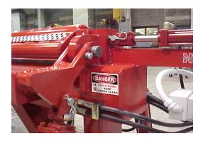
ERMC double benders are built with manual hydraulic controls as standard. The operator is in complete command of the machine.
