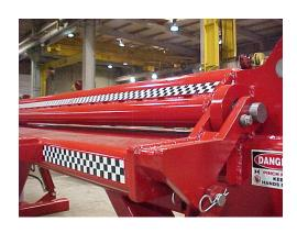
The bending mandrel is safely locked in place by the manually controlled hydraulic locking cylinder. The mandrel is positioned automatically and correctly for each bend.
