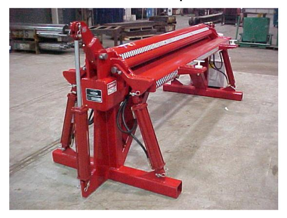
**ERMC Double Benders** were developed in response to the growing precast box culvert market. The standard bender is designed to bend <u>Welded Wire Reinforcing</u> without obstructions in the bending deck through D21 on 2" spacing or D32 on 4" spacing. The radius of the bend is the responsibility of the user, however 2" bending radii will generally conform to the bending specs for precast box culverts (ASTM C-1433). Units are available in 8', 10', and 12' versions.
